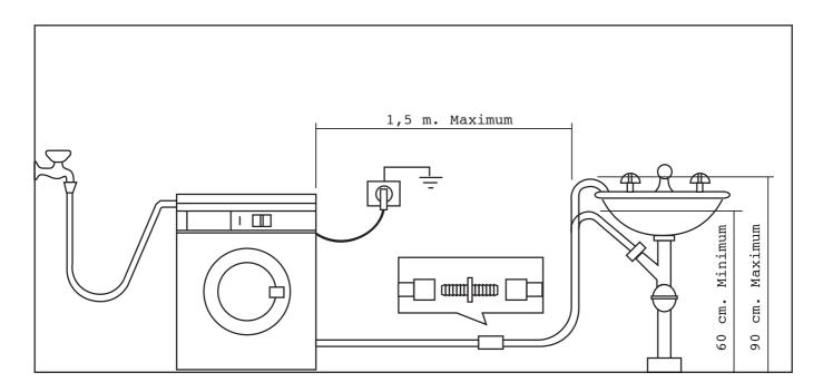
**IMPORTANT:** The distance from the floor to the highest part of the hose should be between 60 to 90 cm. (It is advised to be between 60 and 70 cm). The hose must not be bent nor twisted to avoid clogging. Should a prolongation of the discharging hose be unavoidable this must never surpass 1.5 m and must be of the same diameter as the original hose.
